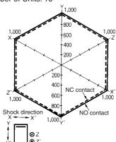
The Units were shocked at the rate of 500 m/s<sup>2</sup> three times each in the  $\pm X$ ,  $\pm Y$ , and  $\pm Z$  directions with and without voltage imposed on the Units until the Units malfunctioned.
