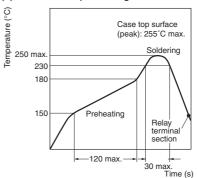
**Note:** The temperature profile indicates the temperature on the relay terminal.
