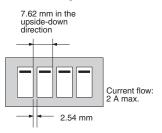
**Note:** The space between relays required for heat radiation may vary with operating conditions. Contact your OMRON representative for details.
