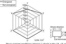
Measurement conditions: Impose a shock in the  $\pm X,\pm Y,$  and  $\pm Z$  directions three times each with the Relay energized to check the shock values that cause the Relay to malfunction.
